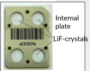
Photons and beta radiation 0.1 – 1000 mSv Photon: Hp(10) and Hp(0.07); 20 keV – 1.3 MeV Beta: Hp(0.07); 0.8 -2.3 MeV
